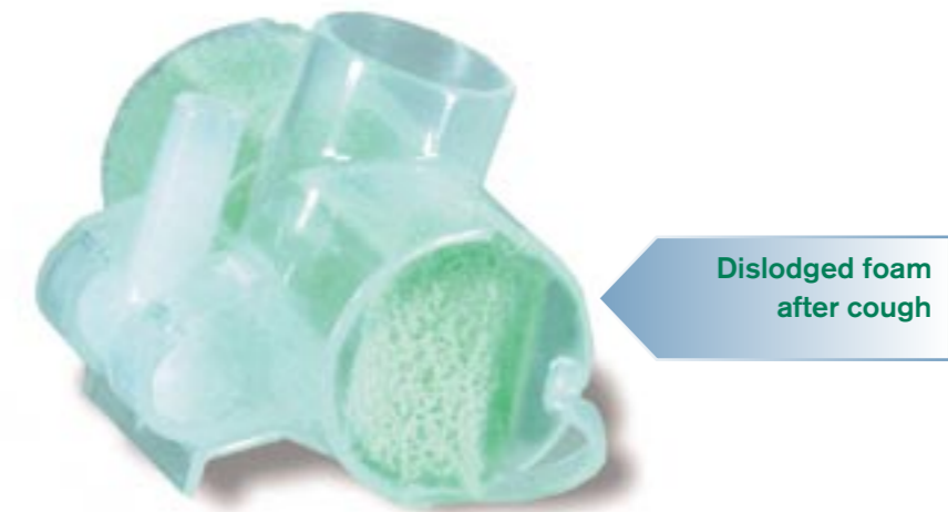
The Hydro-Trach Mk II HME with dislodged foam after a cough.
